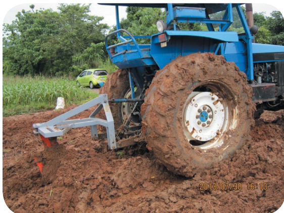
Cassava Digger Prototype tested in muddy terrain using a 90 hp tractor
